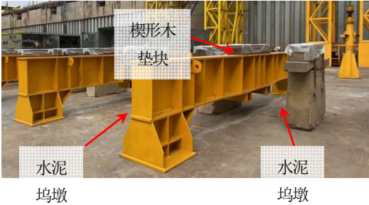
图 13 艏部区域坞墩与门架式支撑工装 Fig. 13 Docking Blocks and Gantry Support Tool at Bow
